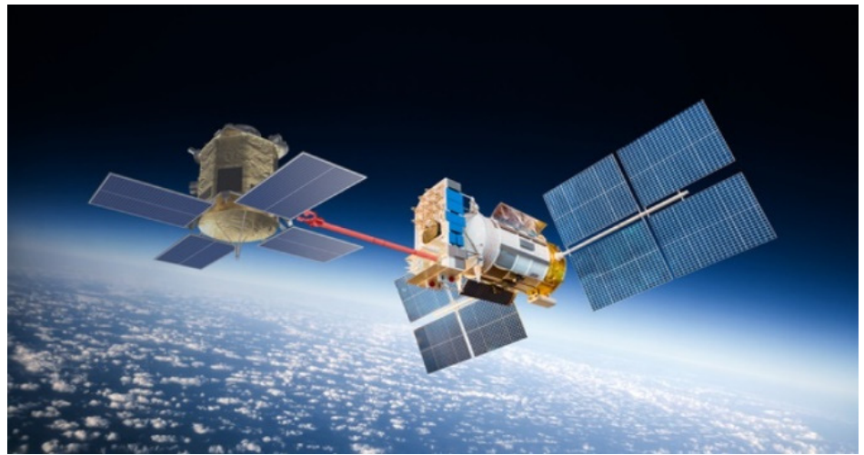
Fig. 33. Illustration of active debris removal (ADR) project using robot arm.
