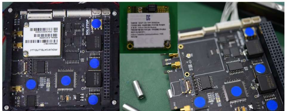
Fig. 8. Failure of iridium module (right) and its original picture (left).
