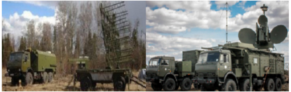
Fig. 9. Russian Electronic Warfare Assets. Russian SATCOM (Satellite Communication) jammer (left) Krashuka-4 jammer (right).
