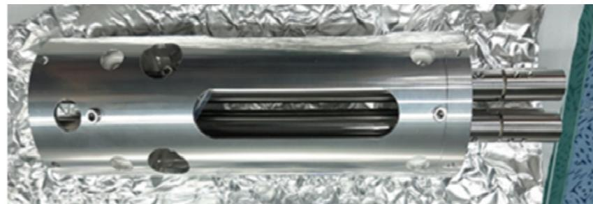
Fig. 9. Prototype quadrupole mass analyzer.
