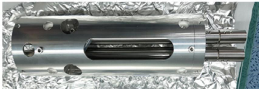
Fig. 9. Prototype quadrupole mass analyzer.
