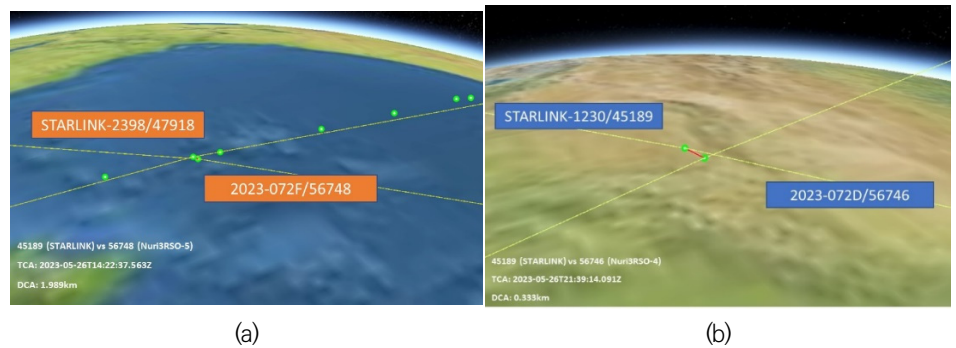
Fig. 10. Visualization of two conjunctions using AstroOne. (a) The Norad ID 56748 satellite is close to the Starlink-2398 satellite having a distance 2 km. (b) The Norad ID 56746 satellite is close to the Starlink-1230 satellite having a distance 0.333 km.
