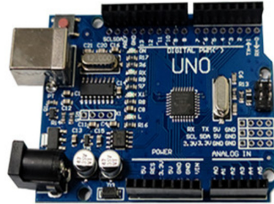
Fig. 7. Arduino Uno R3 compatible board.
