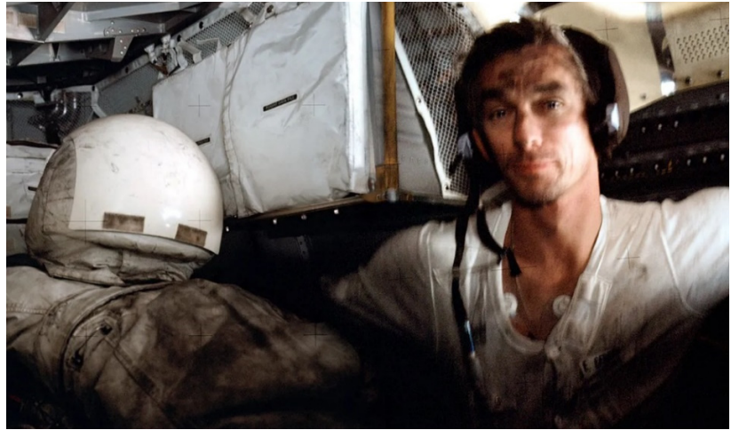
Fig. 6. Crews body surface and spacesuit covered with lunar dust following an extravehicular activity (EVA). Lunar dust can be seen inside the lunar module.
