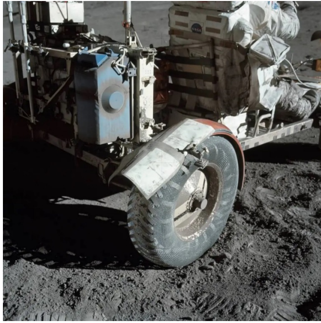
Fig. 4. Lunar dust contamination on the Apollo rover [64].
