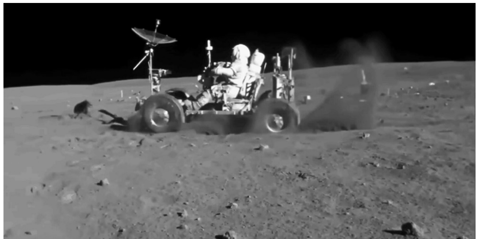
Fig. 3. Lunar dust emission of the Apollo rover [63].
