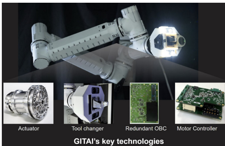
Fig. 24. GITAI Robotic Arm's key technologies.
