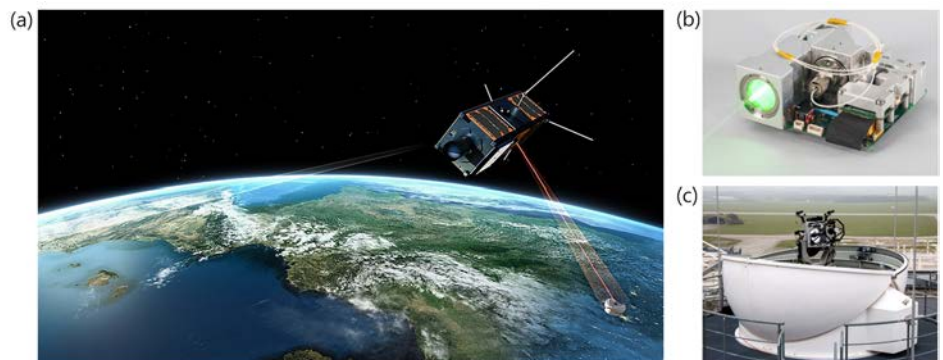
Fig. 1. OSIRIS4CubeSat project: (a) Illustration of optical download from CubeLCT to optical ground station, (b) highly compact laser communication terminal CubeLCT and (c) optical ground station on the roof of the DLR institute of communications and navigation in Oberpfaffenhofen [19]. OSIRIS4CubeSat, Optical Space Infrared Downlink System for CubeSats; DLR, Deutsches Zentrum für Luft- und Raumfahrt.
